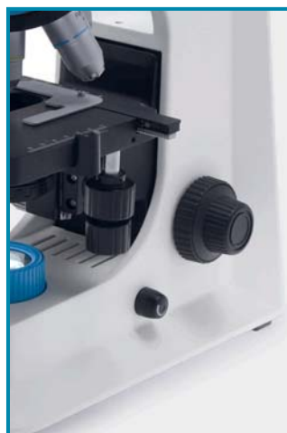
142x138 mm square mechanical stage with 76 mm left-right and 55 mm back-forward movement offers easy use.
