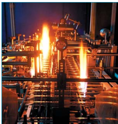
All joints are manufactured by automatic forming machines for consistent quality and guaranteed uniformity.
