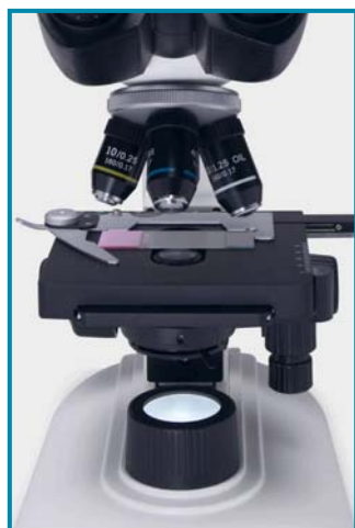
Coarse and fine adjustment is enabled with upper limit safety with 0,002 mm fine division and 20 mm moving limit. Each rotation of control knob enables 42,4 mm coarse stroke and 0,2 mm fine stroke.
