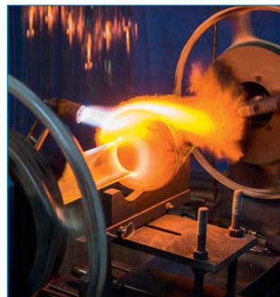
Glass tubes are blown by highly skilled blowers to ensure the uniform wall thickness, exact dimensions according to DIN standards.
