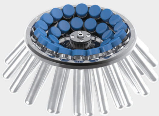
Fix angle rotor for 30 x 15 ml tubes. Max. speed 5000 rpm. Max. RCF 3300 x g. Catalogue no: 603.07.101
