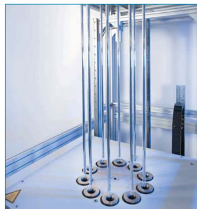
Burette tubings are manufactured by using vacuum technology to maintain diameter of the burette tubings uniform all over their length.
