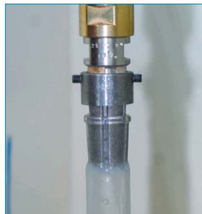
Grinding steps are performed by diamond reamers assuring best results with highest precision.
