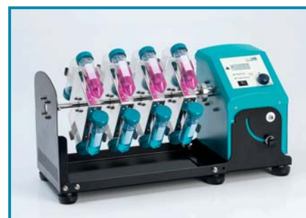
Rotisserie accesory for 50 ml centrifuge tubes hold horizontally.
