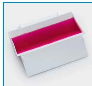
Embossed volume graduations on wall side offers better liquid level viewing and reproducible filling of the reservoir.
