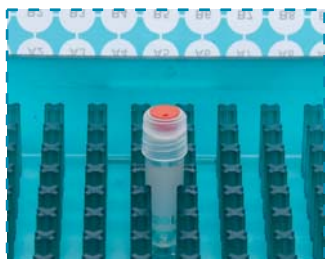
"Hedgehog" designed tube compartments holds the tube in their position firmly.
