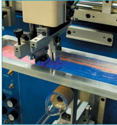
Only high contrasted and fine printing allows precise reading of scaled products such as cylinders, burettes, pipettes etc.
