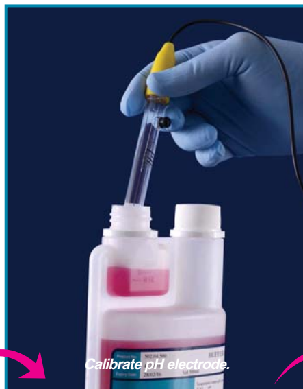
Fill calibration chamber from buffer reservoir by gently pressing the bottle.
