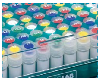
Alphanumerical index both on tube rows and the lid enables easy identification of tube positions.
