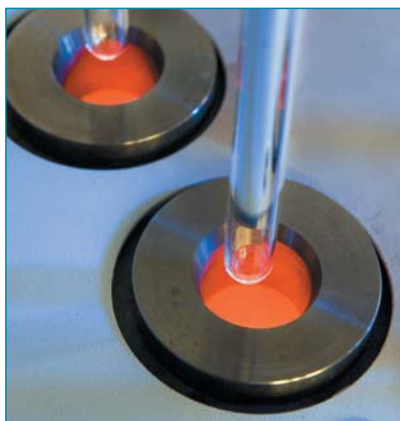
Glass tubings are slowly and gradually heated up to half-melting level. Then they are shrunk around steel rods with precise diameter.
