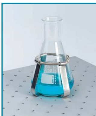
Stainless steel fixing clip adapters for various flasks to be used with clip attachment plate.
