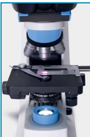
142x138 mm square mechanical stage with 76 mm left-right and 55 mm back-forward movement offers easy use.
