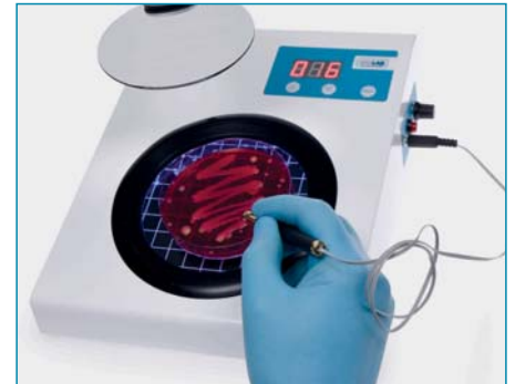
Marking is done by a "felt pin pen" which is connected to the system by cable.
