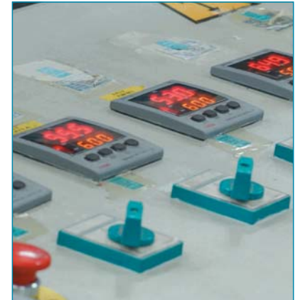
Furnace is entirely controlled by electronic panel for guaranteed temperature control at all steps.
