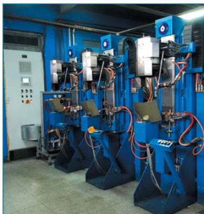
State of the art automatic welding and attaching machines are used for connecting the glass parts to each other.
