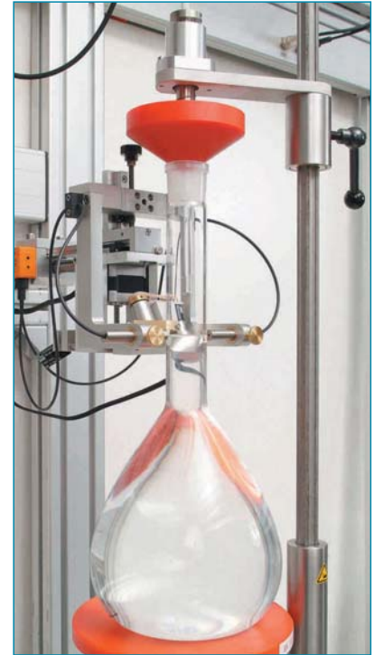
Filling the blank products with water is done automatically by the calibration machines.
