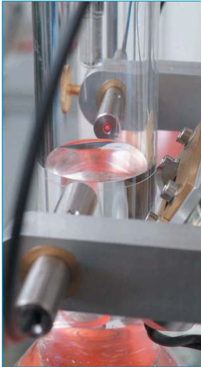
Meniscus is determined automatically at the exact lowest level by a laser beam.
